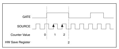
Figure 7-6 shows an example of a single pulse-width measurement.
